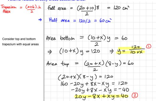
10. A drawing of the cross-section of a skip is shown. The skip company wants to draw a line along the side of the skip indicating half-full.
